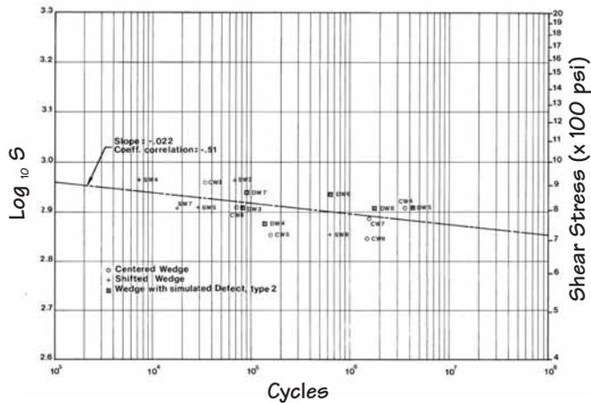
**Figure C-12** S-N Diagram. Longitudinal wedge joint, shear stress, three-point bending tests with Douglas fir/epoxy laminate at room temperature. ( $R=0.1$ , 12% M.C.)
