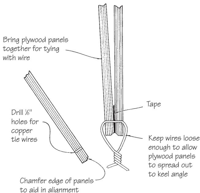
**Figure 25-5** Joining plywood hull panels with wire.
