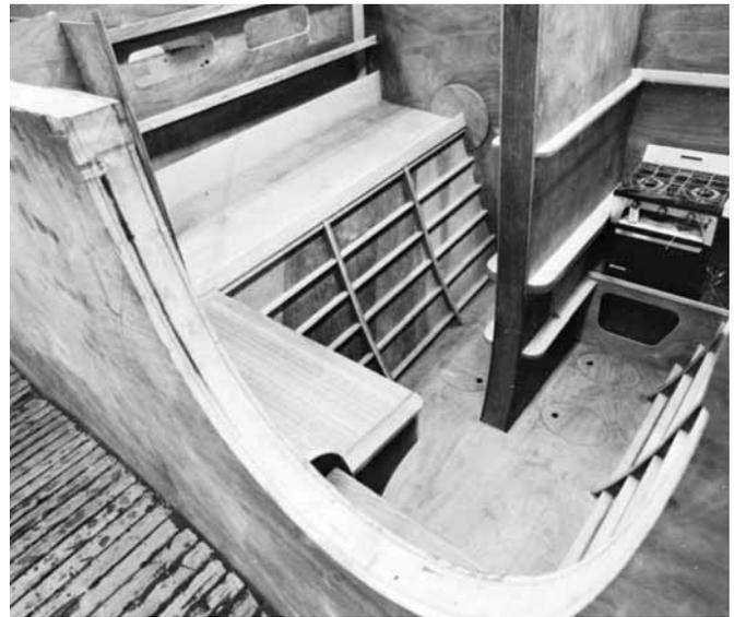
**Figure 26-7** *Rogue Wave's* galley, pilot berth, navigation area, and daggerboard case. All interior joinery was installed before the deck was built. Circular pads on the bulkhead are reinforcing gussets. Note the lift-out access ports in the cabin sole. The unfinished teak cockpit sole is visible at the lower left.
