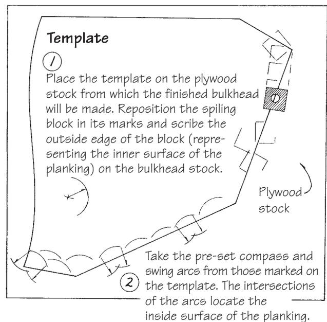
**Figure 26-11** Two methods for transferring the hull shape to a template and then to plywood.
