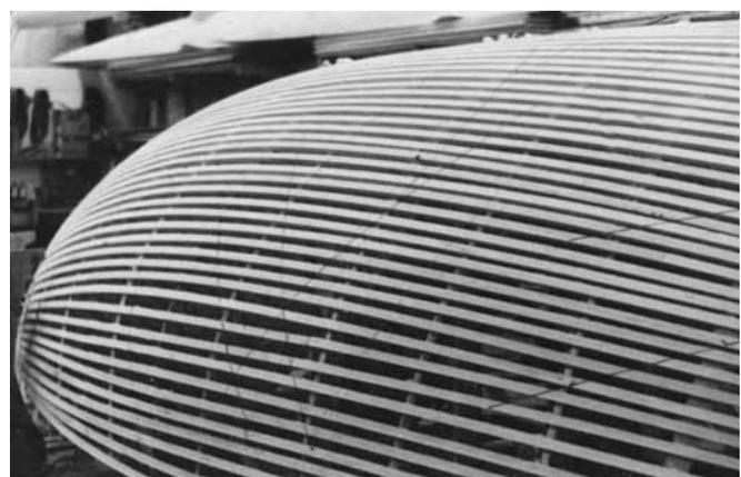
**Figure 21-2** A ribband mold for a 1/2-ton racer showing alignment markings for various veneer layers.
