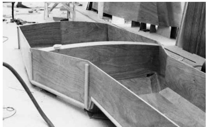
**Figure 27-12** A cockpit assembly constructed outside the hull.
