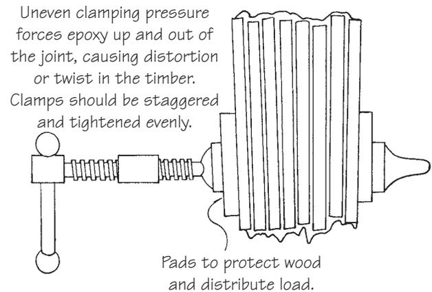
**Figure 11-7** Uneven clamping pressure forces epoxy out of the joint, causing distortion or a twist in the timber. Clamps should be placed in the middle of the laminate, spaced evenly and tightened with consistent pressure.
