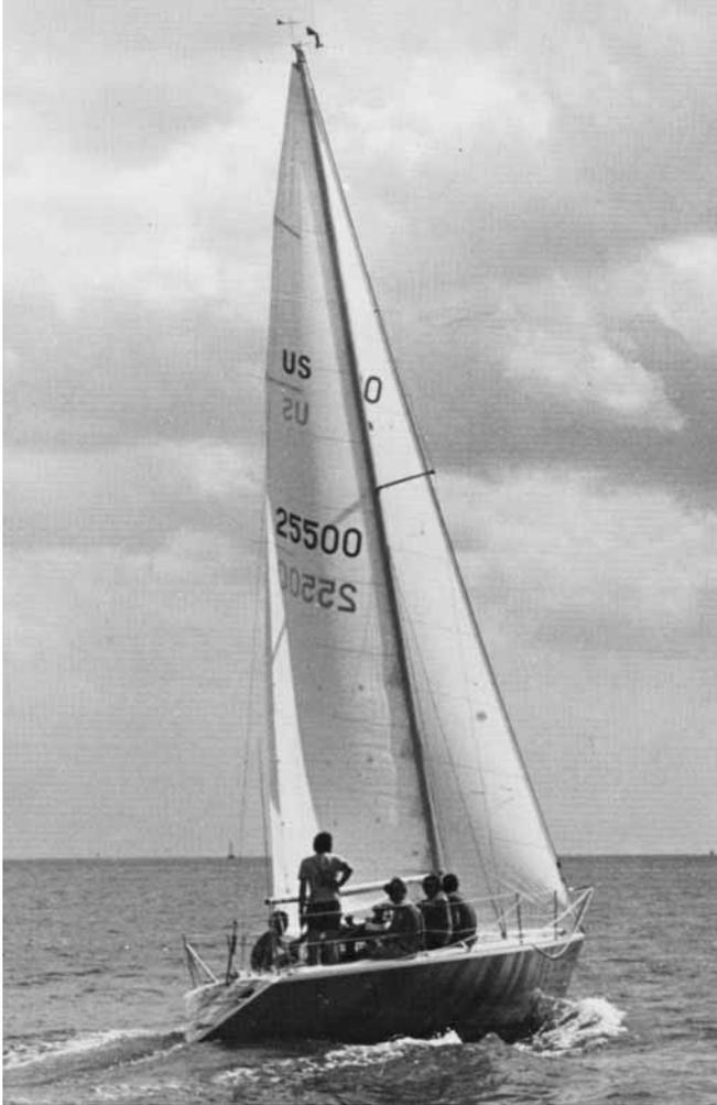
**Figure 5-6** The 32' (9.7m), ½-ton racer *Hot Flash* was built using the stringer-frame method. This type of construction is popular with racing boat designers and builders.
