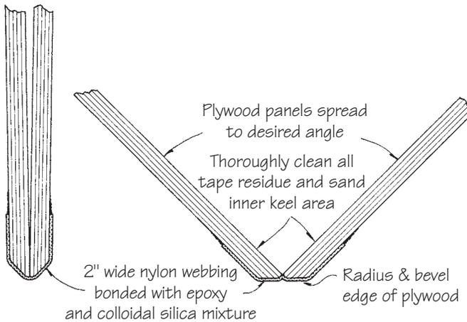
**Figure 25-4** Joining plywood hull panels with nylon webbing.
