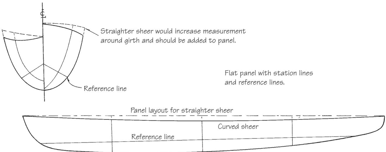
**Figure 25-31** Developing the sheer in a plywood panel layout.
