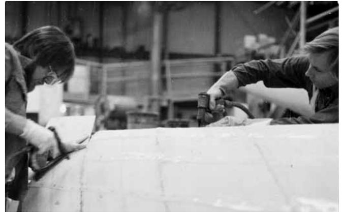
**Figure 21-7** Stapling veneer plank to a hull's stringers. Note the use of plastic strips under the staple heads to ease removal.
