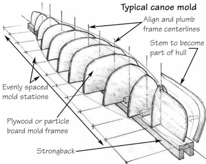
**Figure 23-17** A typical canoe mold with plywood frames.
