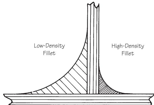
**Figure 11-17** Cross section of low-density and high-density fillets. Low-density fillets require a much larger radius than high-density fillets to make joints of the same strength.
