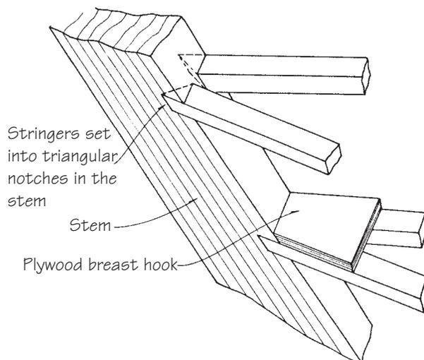
**Figure 22-6** Fitting stringers to a stem or stern post.
