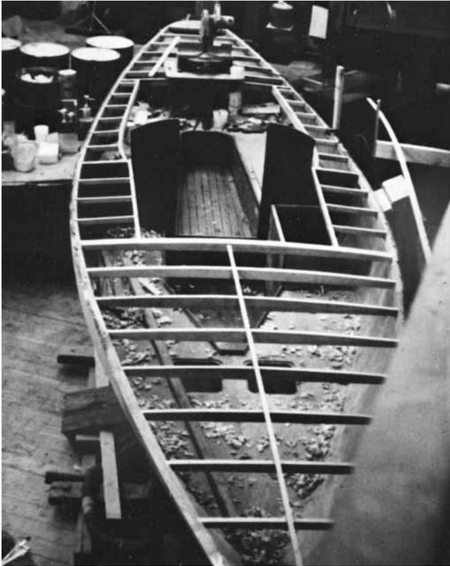
**Figure 27-31** The deck of a 26' (7.9m) Luders 16 framed-in and ready for plywood covering.
