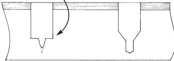
The smaller diameter pilot hole gives the fastener bite into the blocking holding the fastener and fitting until the epoxy cures. You can grind the long tip on the spade bit to avoid drilling through the blocking.
