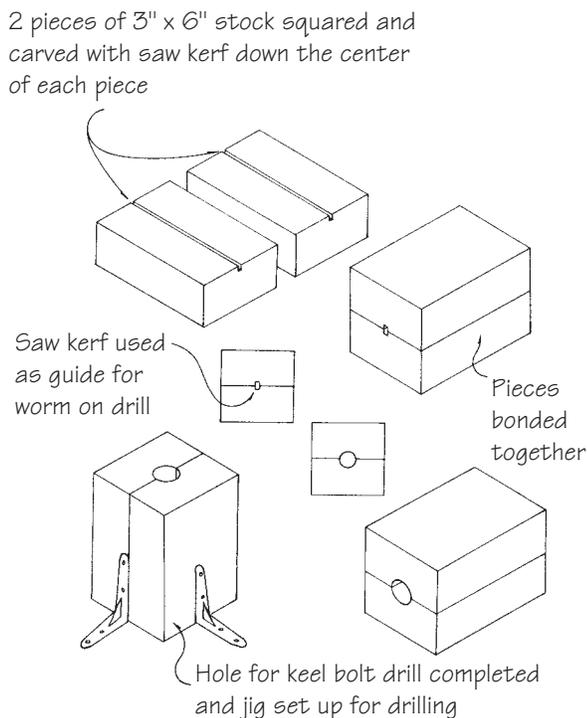
**Figure 14-22** A jig for drilling keel bolt holes.
