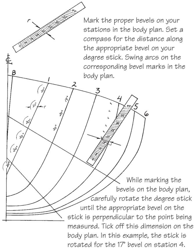
**Figure 16-14** Two methods for subtracting planking thickness for.
