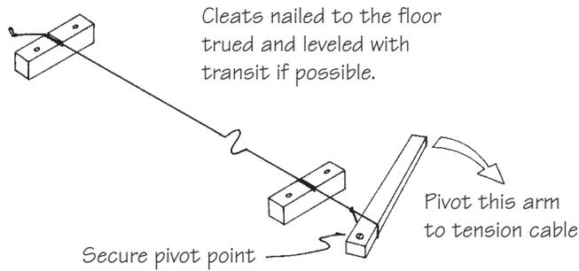
**Figure 16-5** An arrangement for tightening the baseline cable.
