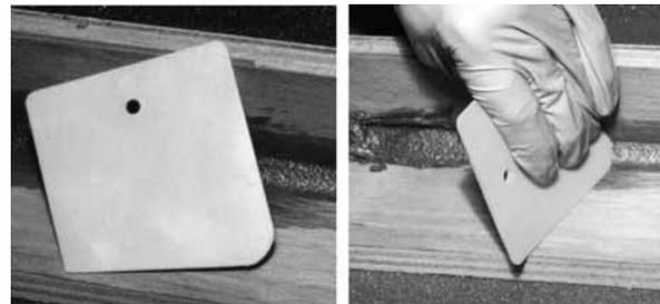
**Figure 11-22** An alternative filleting tool can be made by cutting an 808 Plastic Spreader with the desired fillet radius and the adjoining sides at 75° angle. With an adequate amount of thickened epoxy in the joint and by holding the tool at the proper angle you can make a smooth fillet in one pass. The sides of the tool will force all of the excess epoxy toward the fillet and leave a clean margin on either side.
