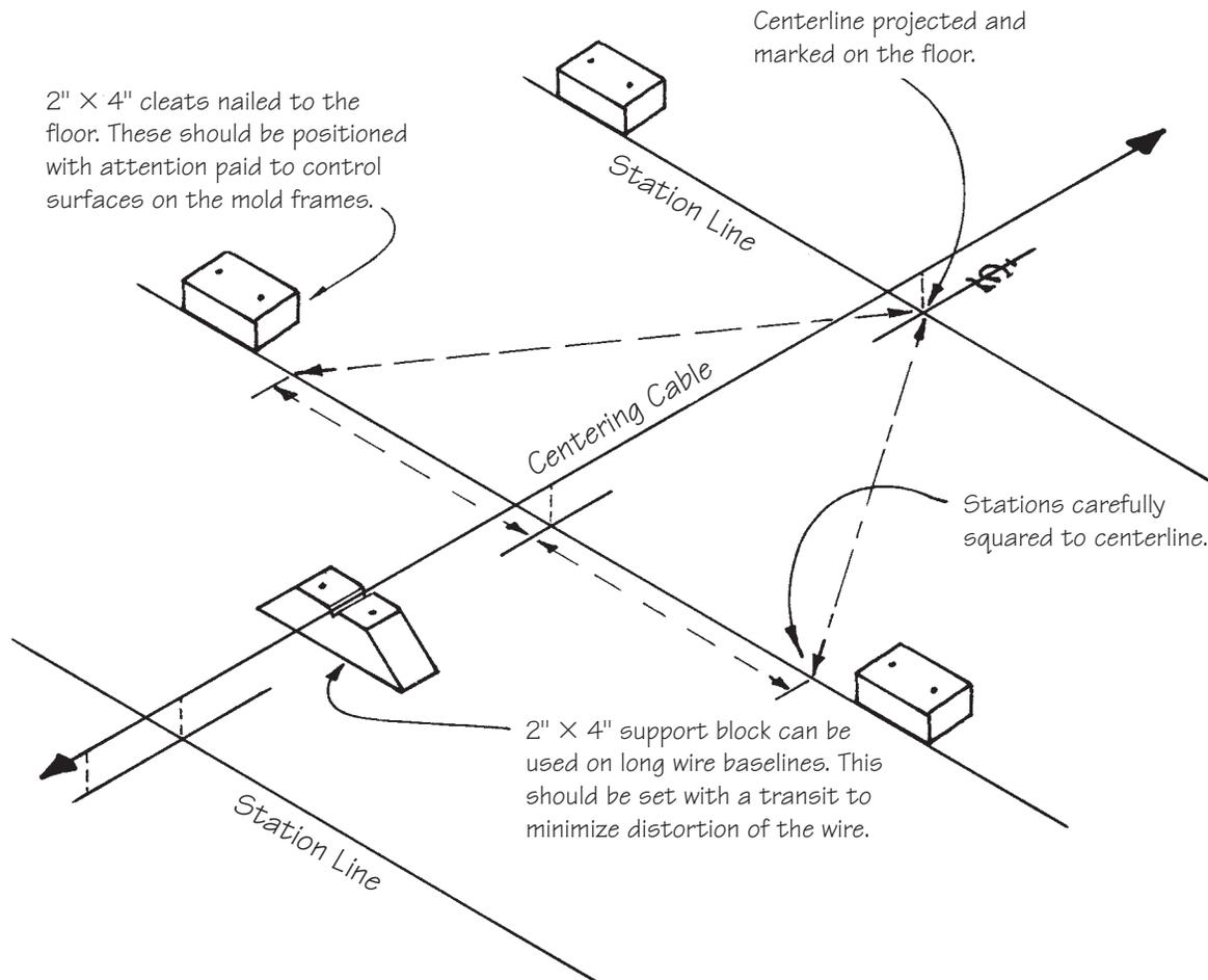
**Figure 18-3** A centering cable and anchor blocks.
