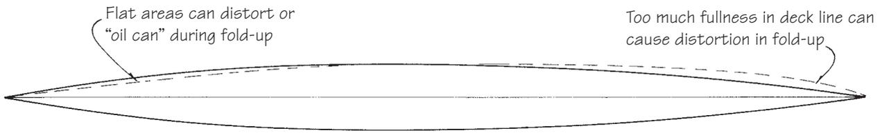
**Figure 25-32** Considerations for deck plans on folded hulls.
