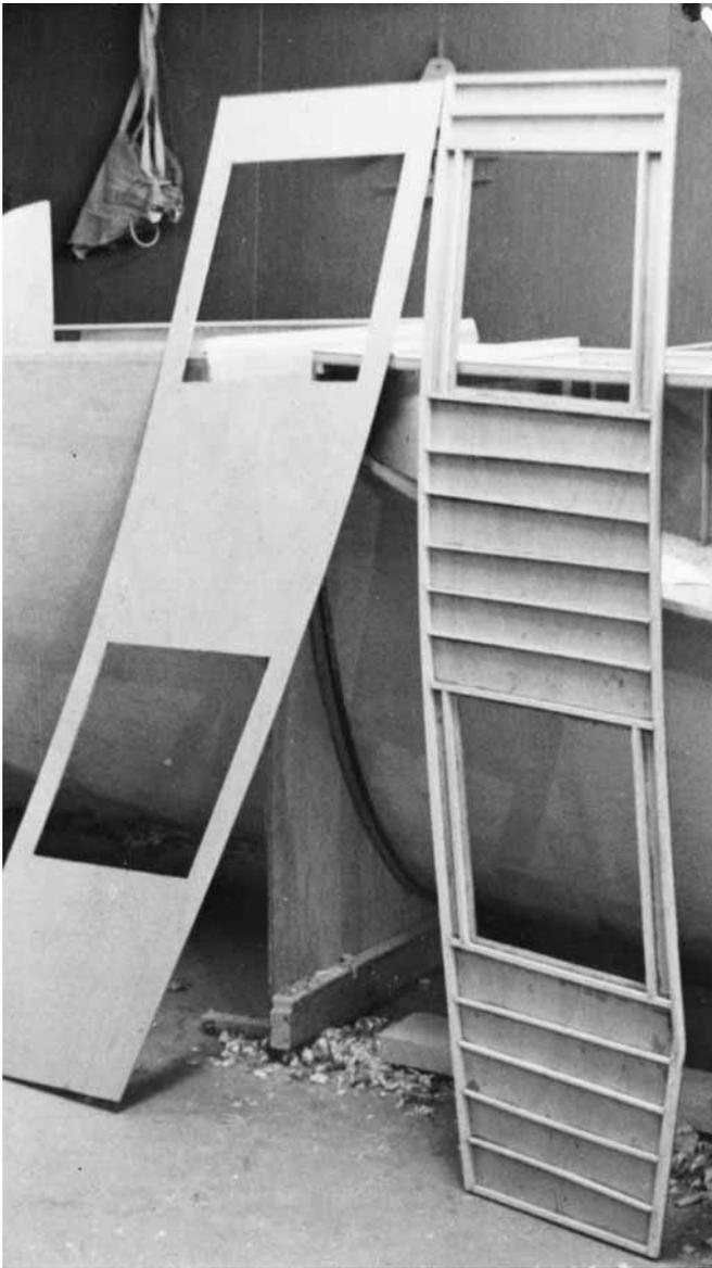
**Figure 11-15** Cockpit seats showing an inner skin bonded to the framing and a matching outer skin. Core material can be cut to fit the spaces within the frames. In this case the framing itself was adequate to support the plywood panels.
