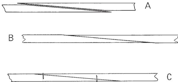
**Figure 12-3** When bonding thin stock or more than one scarf, take care to avoid overmatching the bevels (A) or undermatching the bevels (B). Use wire brads or staples to hold a bevel in proper alignment (C) and prevent slipping during clamping.
