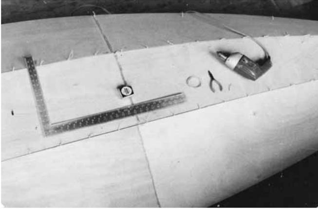
**Figure 24-13** Panel joints of a Fireball dinghy temporarily held with wire. Fiberglass tape will be laid on the inside of these joints and the wires will be removed. After fairing, fiberglass tape or cloth will be applied to the exterior of the joints. (Photo by Mark Lindsay)
