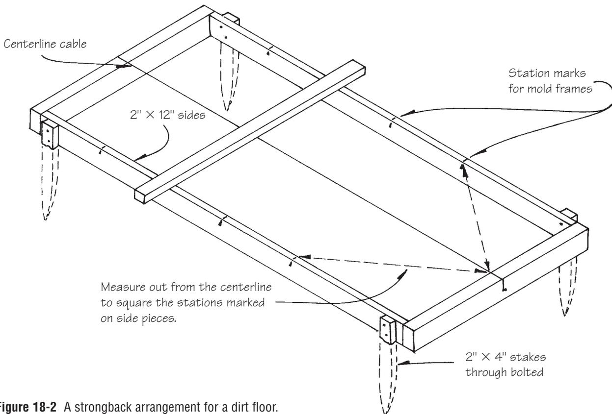
**Figure 18-2** A strongback arrangement for a dirt floor.
