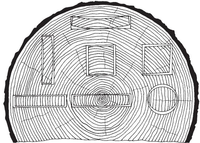
**Figure 3-9** Shrinkage and distortion for wood of various cross sections as affected by the direction of annual rings. Tangential shrinkage is about twice as great as radial. (From *Wood as an Engineering Material*, U.S. Department of Agriculture Handbook, No. 72, p. 3-10.)
