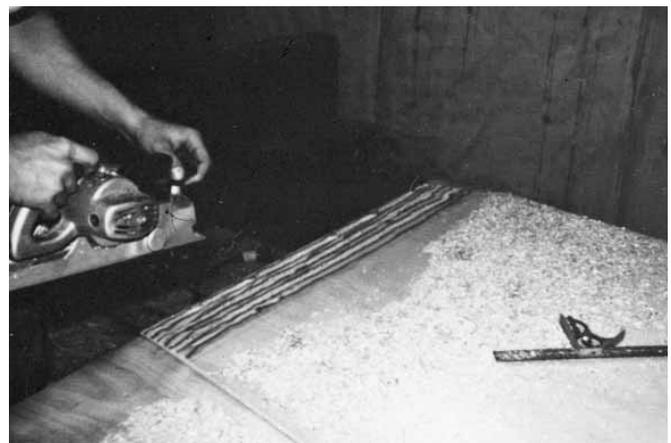
**Figure 12-10** Use a power plane to rough shape a scarf bevel. Finish shaping the bevel with a block plane.
