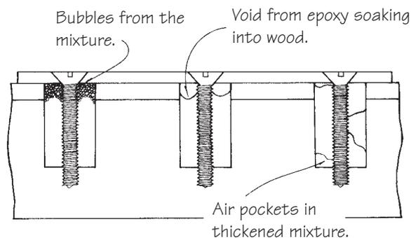
**Figure 14-11** Potential problems with bonded fasteners.
