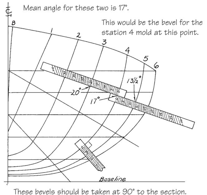
**Figure 16-13** Determining mold bevels using a degree stick.
