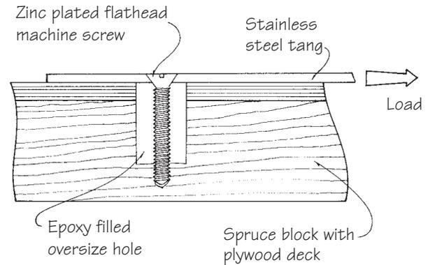
**Figure 14-5** Cross section view of a test sample demonstrating shear load on a fastener.
