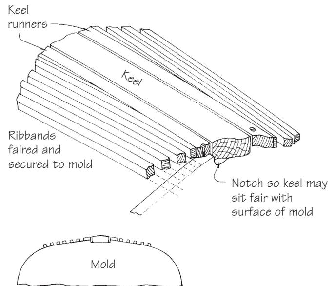
**Figure 20-3** A mold with a recessed keel.
