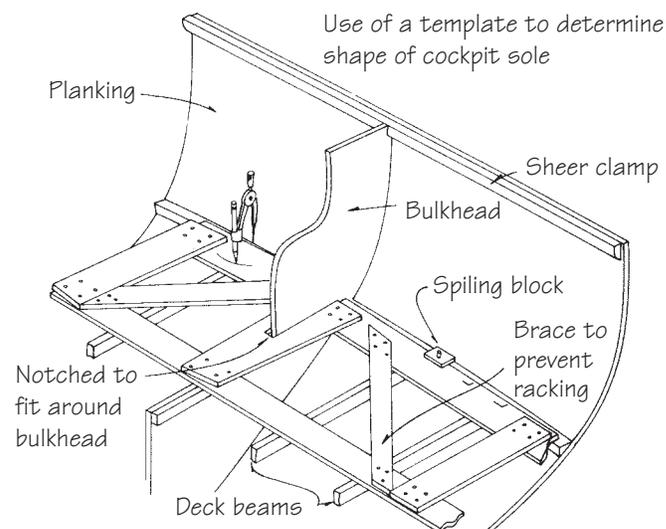
**Figure 26-17** Spiling the shape of a cockpit sole.
