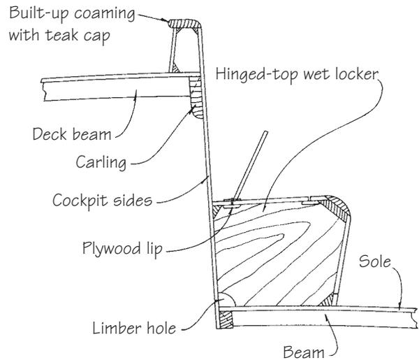
**Figure 27-15** A typical cockpit seat section detail.
