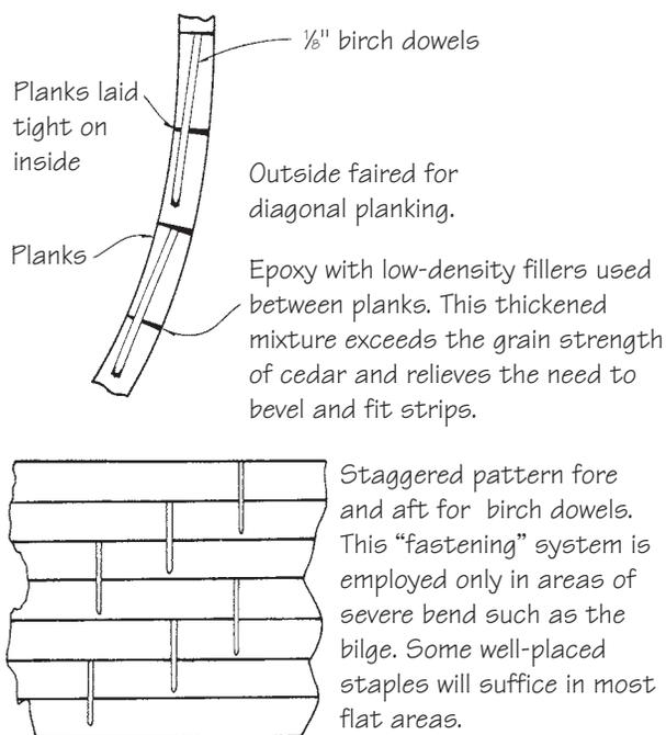
**Figure 23-6** Doweling to prevent plank misalignment.
