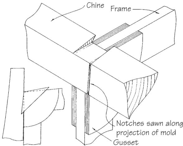
**Figure 24-5** Notching the chine at the frame.
