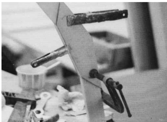
**Figure 17-6** Bonding gussets to permanent frames.
