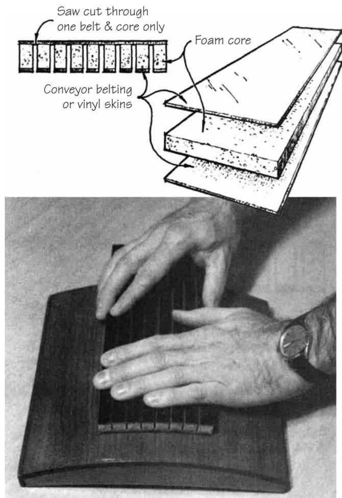
**Figure 23-18** Custom sanding blocks can be made by bonding flexible belting material to a wood or foam core. Vary the core thickness and the saw cut spacing to adjust the flexibility for various curved surfaces.
