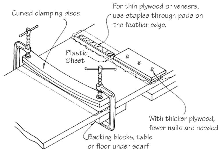
In all cases, use several staples to secure the scarf and prevent slipping during the clamping or nailing operations.
