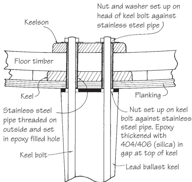
**Figure 14-26** Cross section of a removable bonded keel.
