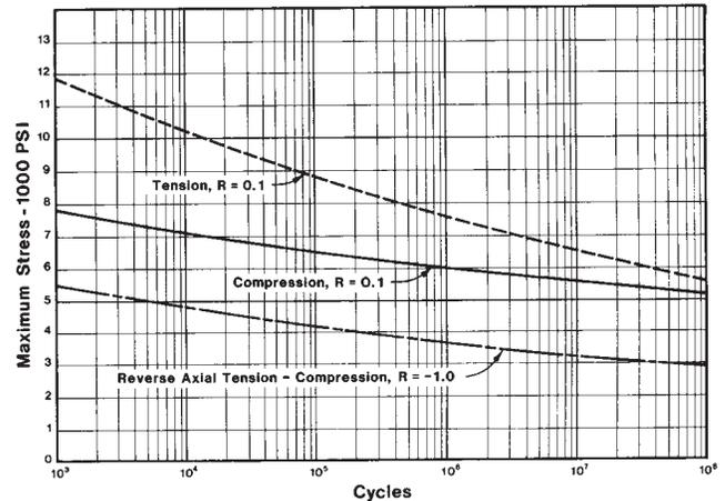
**Figure 3-3** Laminate fatigue properties. Maximum strength adjusted to 12% wood moisture content vs. total cycles for BG-1 Douglas fir/epoxy laminate with 12:1 slope scarf joints with 3" stagger, 31.8 in<sup>3</sup> test volume, parallel to grain load direction, at room temperature.
