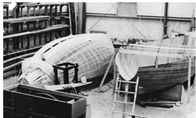
**Figure 21-25** The hull is in a cradle and immediately trued up with the waterlines. Temporary bracing at the sheer stabilizes the shape of the hull while interior joinery is installed. The ladder at the open transom provides easy access to the interior of the hull.
