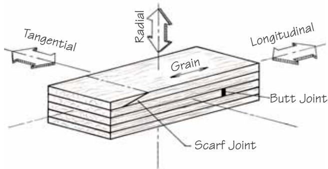
**Figure C-8** Reference axes for laminate strength measurements.
