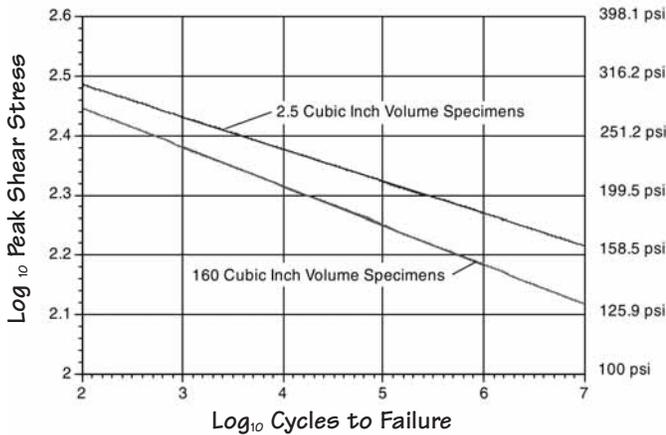
**Figure C-16** Rolling Shear Fatigue Trends for Blade Laminate.
