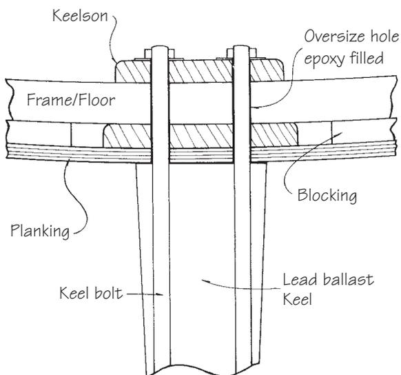
**Figure 14-19** Cross section view of bonded keel bolts.
