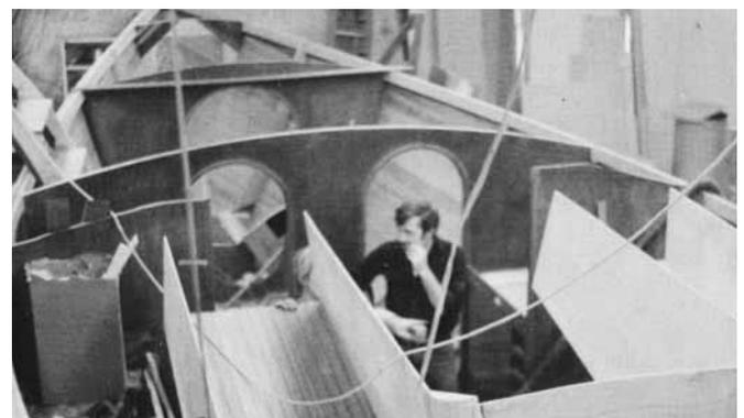
**Figure 27-13** An unusual slingshot-shaped cockpit is set in place on *Golden Dazy*. It is trued up with temporary bracing and blocking. Then the deck framework is installed around its perimeter.
