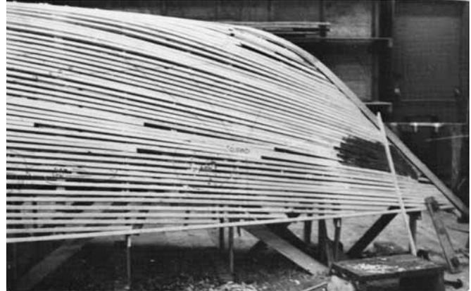
**Figure 20-7** An epoxy/low-density filler mixture was applied near the bow for fairing.
