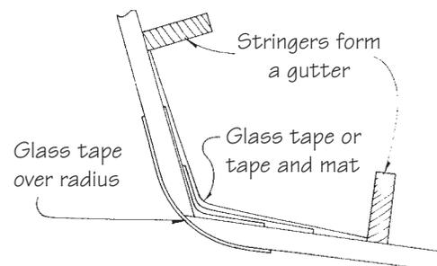
**Figure 24-12** A taped composite chine with conventional stringers.
