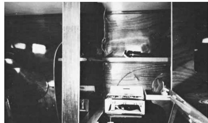
**Figure 26-8** *Rogue Wave's* galley area after the deck was installed. Sandwich construction of the deck in this area required a headliner skin. This smooth plywood panel was painted white to lighten the naturally finished interior.
