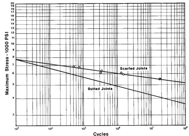
**Figure 3-4** Compression fatigue. Maximum stress vs. total cycles for Douglas fir/epoxy laminate with 12:1 slope scarf and butt joints with 3" stagger, 31.8 in<sup>3</sup> test volume, parallel to grain direction, room temperature and 12% wood moisture content.
