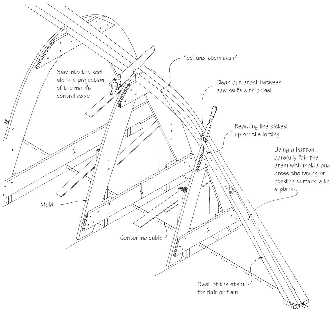
**Figure 19-7** A set-up for a typical IOR racer. Control lines have been drawn on the stem. Notches are cut in the keel at the molds to determine bevels. The stem is blocked up to allow the centerline cable to pass freely underneath.
