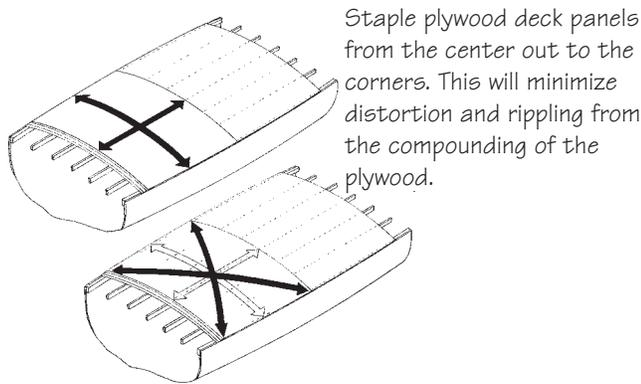
Staple plywood deck panels from the center out to the corners. This will minimize distortion and rippling from the compounding of the plywood.
