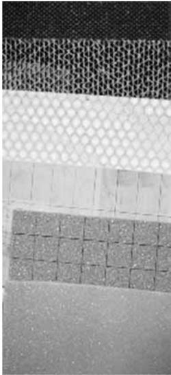
In sandwich construction, fiber reinforced resin serves as the structural skin of a part. Separating two structural skins with a core material will improve the composite's stiffness and reduce weight, much like the web of an I-beam separates the flanges. Cores can be of plywood, end-grain balsa, foam or honeycomb. Normally, the core is much lighter than the skin material. Like most materials, different cores have advantages and disadvantages.
