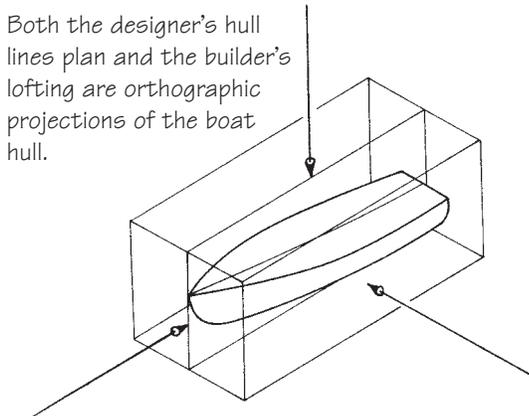
**Figure 16-1** The lines show three different views of the boat. The amateur builder will find the building project much easier if he takes the time to study the plans and attempts to see the boat in the lines.
