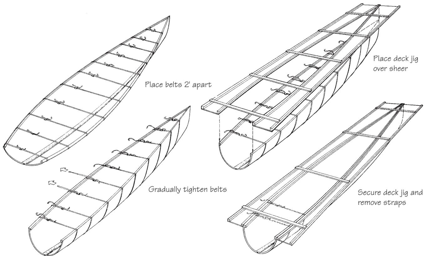
**Figure 25-13** Folding up with plastic strapping or belts.
