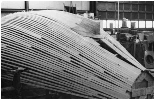
**Figure 20-6** A ribband mold for an IOR ½ ton racer. Note the use of shorter ribbands to fill gaps between full-length ribbands. The skeg shown was laminated out of veneers beforehand, then secured to the mold. The veneer used to plank the hull was bonded to the skeg. This was done to save the extra expense and time of molding such an extreme shape during general laminating.
