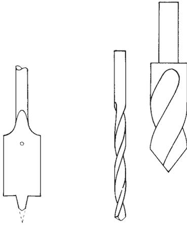
Any drill will do; however, the spade bit will give you more major diameter surface area for a given hole depth because of the square cut.
