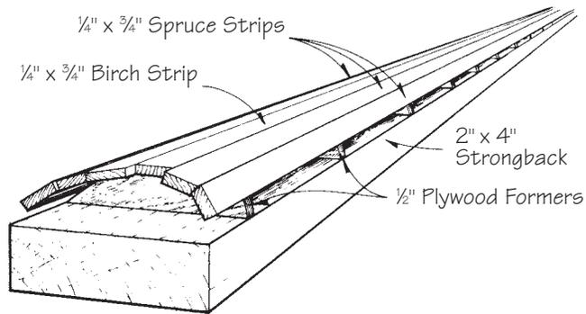
**Figure 23-19** Building a strip composite spar.
