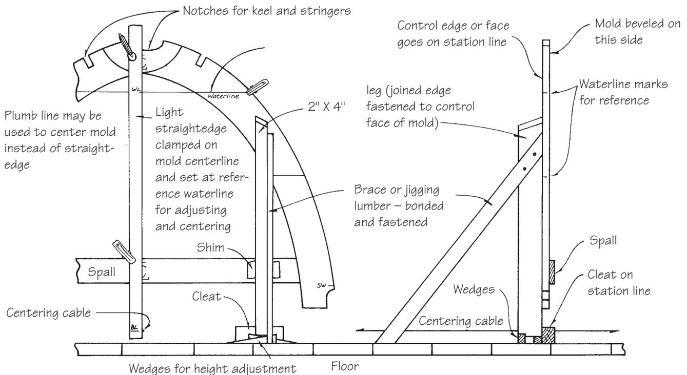
**Figure 18-5** Two views of a typical frame set.
