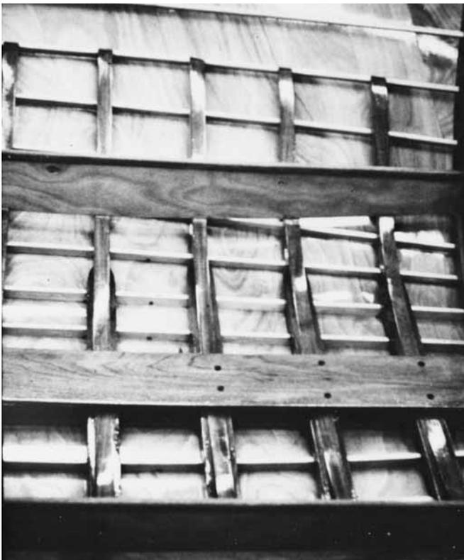
**Figure 26-27** Prefinished interior on an IOR ½ ton racer.
