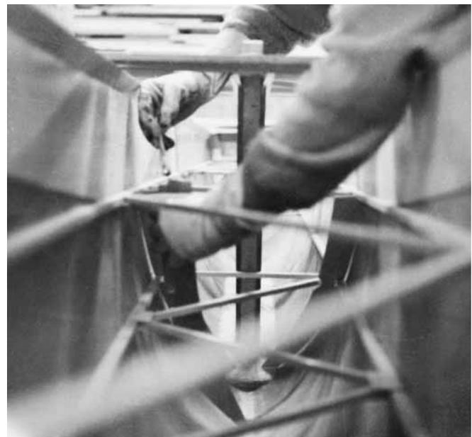
**Figure 25-17** Struts and bracing for sub-level stringers in a Tornador catamaran hull. Note the small plywood gussets holding the struts to the stringers. Small plywood half frames are being installed against the hull skin. These frames will be filleted to the skin. The centerboard case is the vertical structure in the middle of the hull.
