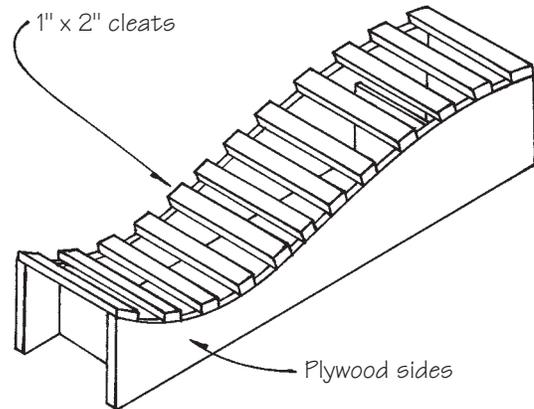
**Figure 11-3** A simple form for laminating wider pieces.
