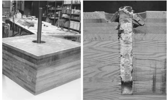
**Figure 14-4** The  $1\frac{1}{2}$ " test samples before testing (left) and a cutaway of the damage after testing (right). The  $1\frac{1}{2}$ " silicon bronze threaded rods were imbedded perpendicular to the glue joints.
