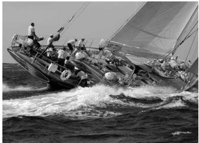
**Figure 5-4** The 124' (37.7m), Bruce King designed, sloop *Antonisa* was built by Hodgdon Yachts, Inc. using the strip plank/veneer method. Hulls as large as 213' (65m) have been built with this method.
