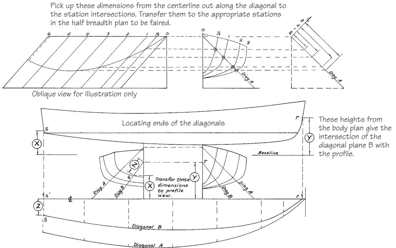
**Figure 16-9** Laying off diagonals.
