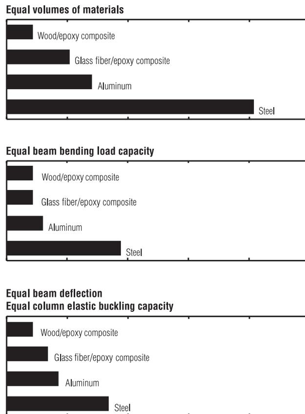
**Figure 3-7** Relative weights of flat panels built with various structural materials. Wood/epoxy composite built with ultrasonically graded Douglas fir and WEST SYSTEM epoxy.
