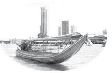
or truck engine mounted on a pedestal at the rear. A long propeller shaft leads from the engine into the water. These are called long tailed boats. They are quite fast and roar across the river raising a tall "rooster tail" of water. You will get an exciting ride but you must know where you want to get off and signal the driver when approaching your destination since they do not automatically stop at every landing.
