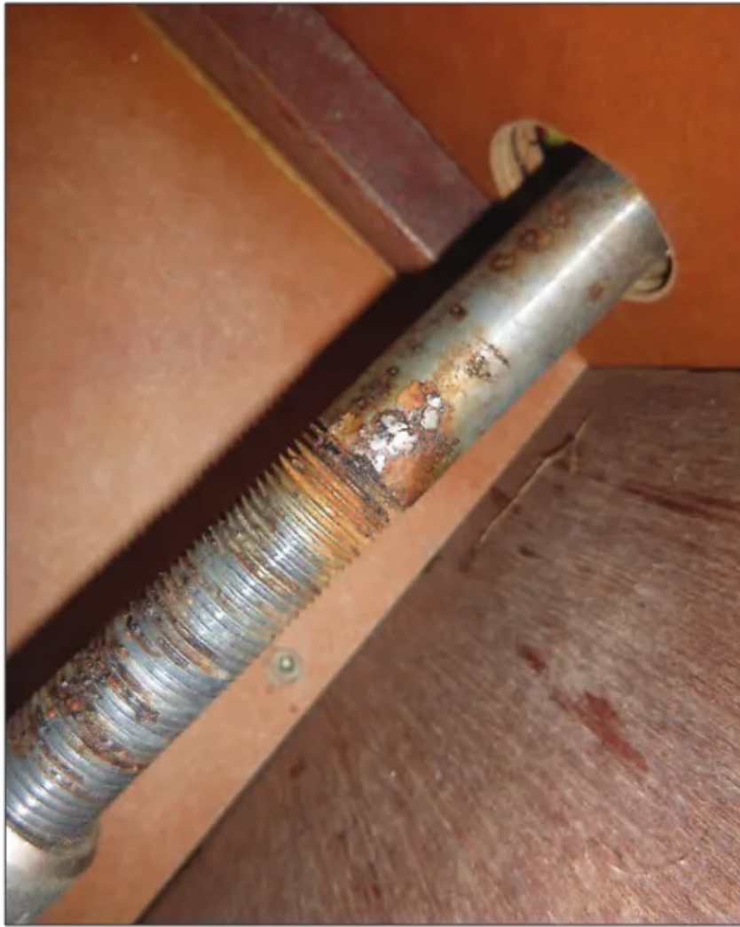
Left —For rod attachments, in addition to inspecting the plate that affixes to the hull, sight down the rod itself for signs of corrosion. Above —Dye-penetrant testing requires thorough cleaning of the metal before applying dye and developer to expose the smallest cracks and pits.
