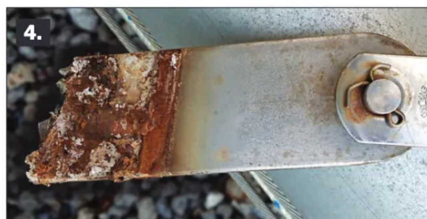
1 —Take photographs with a camera set on macro and then magnify them on a computer screen to reveal cracks missed by a visual inspection in the field. 2 —Remove surface rust with a nylon scouring pad to show any underlying pits and cracks. 3 —Small cracks or rust blooms on the edges of a plate likely indicate greater problems between the stainless steel and the hull. 4 —A chainplate may appear sound at the rig attachment point but be entirely destroyed under the deck where moisture was held against it without oxygen.
