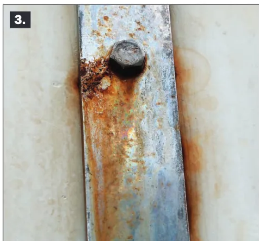
1 —Take photographs with a camera set on macro and then magnify them on a computer screen to reveal cracks missed by a visual inspection in the field. 2 —Remove surface rust with a nylon scouring pad to show any underlying pits and cracks. 3 —Small cracks or rust blooms on the edges of a plate likely indicate greater problems between the stainless steel and the hull. 4 —A chainplate may appear sound at the rig attachment point but be entirely destroyed under the deck where moisture was held against it without oxygen.
