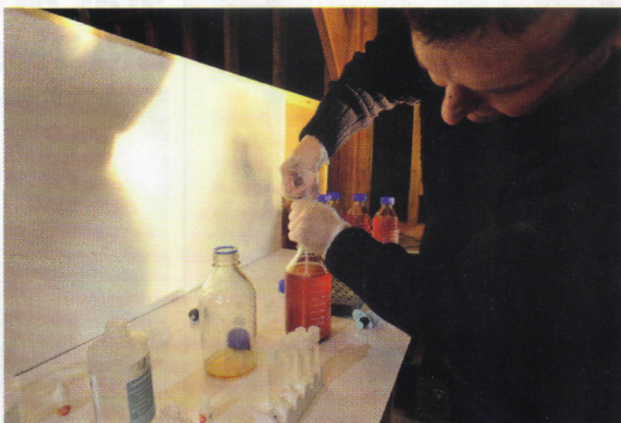
1 Draw a sample of contaminated fuel into a syringe from the interface between the fuel and water – this is where the diesel bug will be found.
