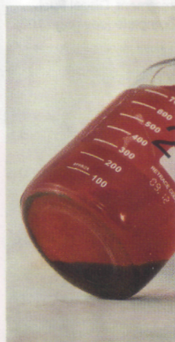
Deposits and poor dispersal suggest inadequate dosing
