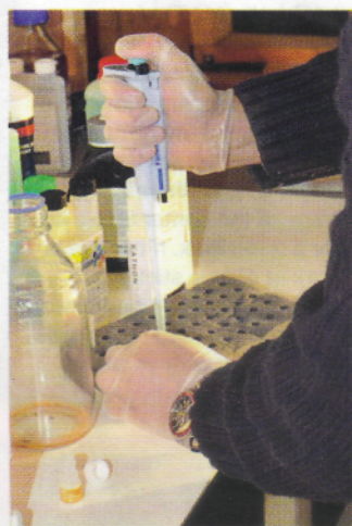
6 Transfer a measured amount of fluid from the extraction tube to a culture tube and add two drops of the enzyme luciferase.
