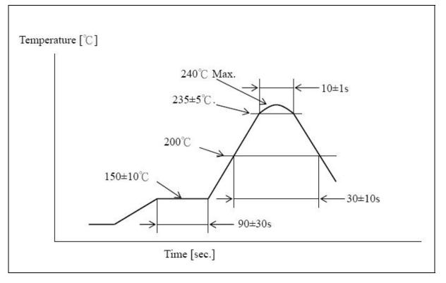
Pre heating temperature: $150\pm10[^{\circ}C]$ Pre heating time: $90\pm30[sec.]$ Heating temperature: $235\pm5[^{\circ}C]$ Heating time: $10\pm1[sec.]$ Peak temperature must not exceed 240°C and the duration of over 200°C should be  $30\pm10$ Seconds.
