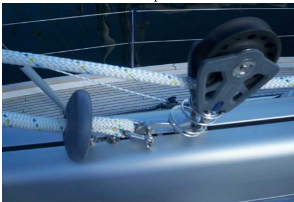
Wrong position – will scratch the boom
