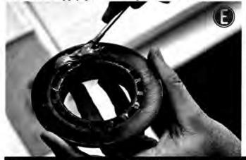
E: Apply a good layer of mixed glue all over the roughened base of the flange, again making sure you don't get any on the thread. You have quite a while before it starts to cure so take your time!
