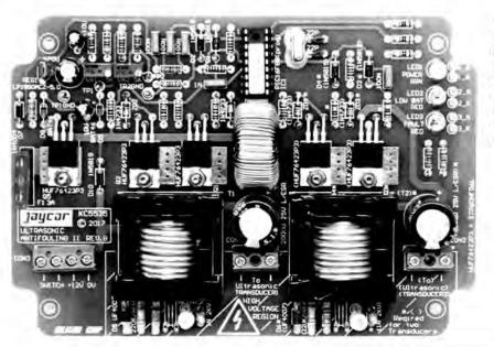
The Ultrasonic Anti-Fouling Unit can be built to drive one or (as shown here) two ultrasonic transducers. If your craft is less than 8m long, you should be able to get away with one – in which case, the majority of components on the bottom right of this photo are not installed (see below).
