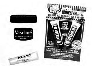
You'll need each of these to mount the transducers in your boat: some Vaseline (petroleum jelly), some Fix-a-tap waterproof lubricant (available at plumbing suppliers) and some J-B Weld two-part epoxy (available at Jaycar stores). We do not recommend any other epoxy glues – J-B Weld really holds on even with a boat hull's vibration and stress!
