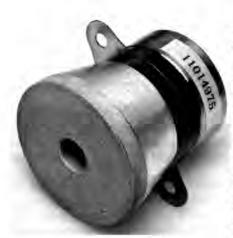
(Left): here's the "business end" of the system, the Ultrasonic Transducer, which sets up the vibration pattern in the boat hull which marine vegetation doesn't particularly enjoy! Because these operate at high voltage (~700-800V peakto-peak) they must be fully enclosed ("potted") in a suitable enclosure, as shown above. (The
