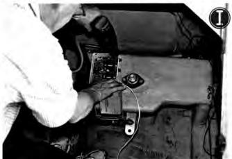
If you can run the cable next to existing cable, so much the better. Lace or tie the cable into position where possible. It should not be allowed to flap about or hang in loose loops.
