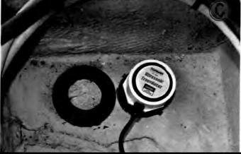
C: Move the empty flange around the hull to determine the best transducer mounting position. When you're happy with your choice, roughen the surface as you did the black flange – for the same reason.
