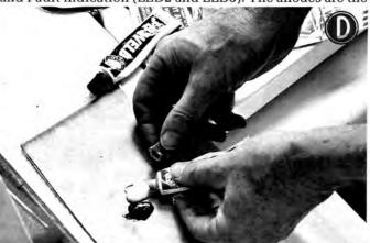
D: We're recommending J-B Weld to secure the flange to the hull. It's not that easy to buy (but Jaycar stores do stock it – Cat NA1518) and it's not real cheap – but it sticks like the proverbial.
