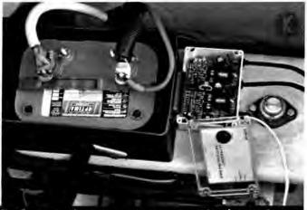
K: after mounting, connect to an appropriate battery (one that receives shore power or solar panel charging). Dress the leads so that they can't move around (remember that there is severe vibration present).
