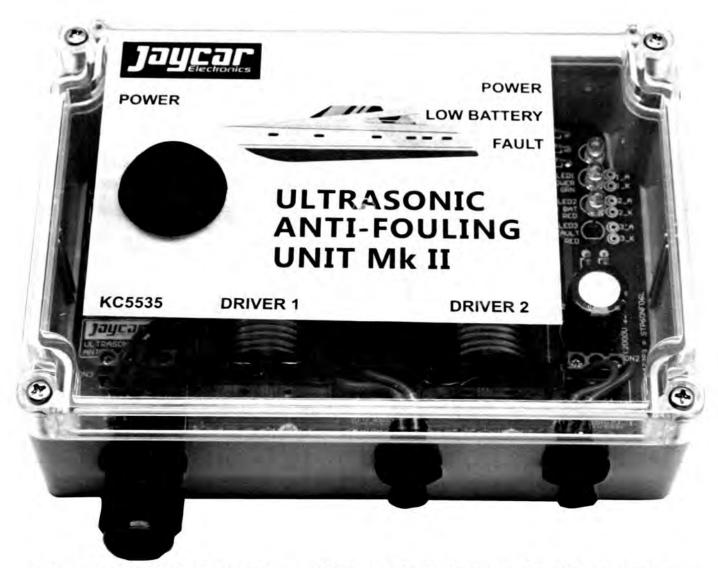
... and here it is with the lid fitted, with the front panel label mounted inside for protection from the marine environment.
